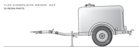
Anhängerfahrgestell A 1 - the type A1 single-axle light trailer chassis - had been designed for Luftwaffe before the war, . It had a weigh of 140 kg, and payload of 610 kg (750 kg - for type A1B), and was to be towed by light motor vehicles, or even by men power. The construction was very simple, yet, the A1 was used as chassis for many superstructures and auxiliary trailers.
